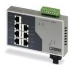
Ethernet Switch, 7 TP RJ45 ports, 1 FO port, 100 Mbps full duplex in SC-D format, automatic detection of data transmission speed of 10 or 100 Mbps (RJ45), autocrossing function
