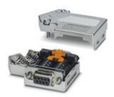
D-SUB connector, 9-pos. socket, 35° cable entry, bus system: CAN, CANopen<sup>®</sup>, SafetyBUS p up to 1 Mbps, with PG D-SUB socket for connecting a programming device, termination resistor can be switched on via slide switch, pin assignment: 2, 3, 7, 9; screw terminal blocks
