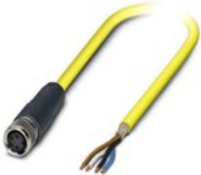
Sensor/actuator cable, 4-position, PVC, yellow, shielded, free cable end, on Socket straight M8, cable length: 5 m
