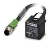
Sensor/actuator cable, 5-position, PUR halogen-free, black-gray RAL 7021, Plug straight M12 SPEEDCON, coding: A, on Valve connector AD (pressure switch), with 2 LEDs, cable length: 0.6 m
