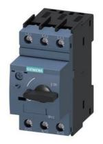
Circuit breaker size S0 for system protection without phase failure protection A-release 2.8...4 A Short-circuit release 52 A Screw terminal Standard switching capacity
