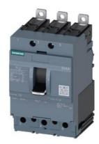
circuit breaker 3VA4 UL frame 125 breaking capacity class M 35kA @ 480 V 3-pole, line protection TM210, FTFM, In=100A overload protection Ir=100A fixed short-circuit protection Ii=10 x In clamp connection
