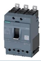
circuit breaker 3VA4 UL frame 125 breaking capacity class S 25kA @ 480 V 3-pole, line protection TM210, FTFM, In=60A overload protection Ir=60A fixed short-circuit protection Ii=10 x In clamp connection
