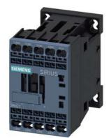
coupling contactor relay, 2 NO + 2 NC, 36 V DC, 0.7-1.25\* Us, with integrated varistor, spring-loaded terminal, frame size S00, suitable for PLC outputs, not expandable with auxiliary switch expandable
