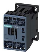
coupling contactor relay, 4 NO, 36 V DC, 0.7-1.25\* Us, with integrated varistor, spring-loaded terminal, frame size S00, suitable for PLC outputs, not expandable with auxiliary switch expandable
