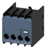
auxiliary switch, on the front, 2 NC, 71/72, 81/82, current path: 1 NC, 1 NC, cable entry from below, screw terminal, for contactors 3RT2 and contactor relays 3RH2
