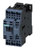
power contactor, AC-3e/AC-3, 32 A, 15 kW / 400 V, 3-pole, 125 V DC, 0.7-1.25\* Us, with plugged-in varistor, auxiliary contacts: 1 NO + 1 NC, spring-loaded terminal, size: S0, suitable for PLC outputs, not expandable with auxiliary switch
