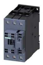
power contactor, AC-3e/AC-3, 65 A, 30 kW / 400 V, 3-pole, 230 V AC, 50/60 Hz, with plugged-in RC element, auxiliary contacts: 1 NO + 1 NC, main circuit: screw terminal, control and auxiliary circuit: spring-loaded terminal, size: S2,
