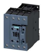
power contactor, AC-3, 41 A, 22 kW / 400 V, 4-pole, 48 V AC, 50/60 Hz, main contacts: 2 NO + 2 NC, auxiliary contacts: 1 NO + 1 NC, screw terminal, size: S2
