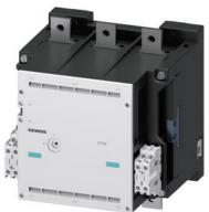
vacuum contactor AC-3e/AC-3 630 A, 335 kW / 400 V, Ue 690 V, 3-pole, Uc: 110-132 V AC(50/60 Hz) drive: conventional auxiliary contacts 4 NO + 4 NC main circuit: busbar control and auxiliary circuit: screw terminal
