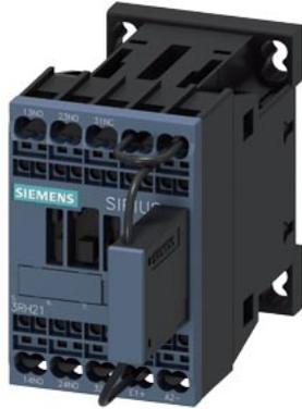
contactor relay railway, 2 NO + 1 NC, 220 V DC, 0.7-1.25\* Us, with integrated suppressor diode, spring-loaded terminal, frame size S00
