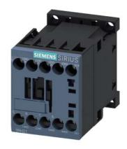
contactor relay railway, 3 NO + 1 NC, 72-125 V DC, 0.7-1.25\* Us, with integrated varistor, screw terminal, frame size S00  $\,$
