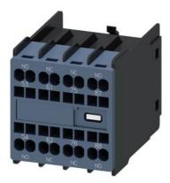
auxiliary switch, on the front, 2 NO + 2 NC, 11 U, 53/54, 61/62, 75/76, 87/88, current path: 1 NO, 1 NC, 1 NC (lagging), 1 NO (leading), spring-loaded terminal, for contactors 3RT2 and contactor relays 3RH2
