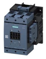
power contactor, AC-3e/AC-3 150 A, 75 kW / 400 V AC (50-60 Hz) / DC Uc: 23-26 V 3-pole, auxiliary contacts 2 NO + 2 NC drive: conventional main circuit: box terminal control and auxiliary circuit: screw terminal box terminal up to 70  $\,\mathrm{mm^2}$
