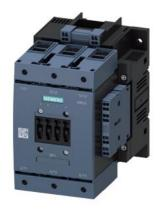
power contactor, AC-3e/AC-3 185 A, 90 kW / 400 V AC (50-60 Hz) / DC Uc: 23-26 V 3-pole, auxiliary contacts 2 NO + 2 NC drive: conventional main circuit: box terminal control and auxiliary circuit: screw terminal box terminal up to 70  $\,\mathrm{mm^2}$
