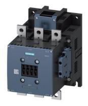
power contactor, AC-3 300 A, 160 kW / 400 V, AC (50-60 Hz) / DC operation 110-127 V AC/DC auxiliary contacts 2 NO + 2 NC 3-pole, frame size S10 busbar connections drive: conventional screw terminal NEMA version
