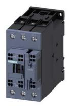
power contactor, AC-3e/AC-3, 41 A, 18.5 kW / 400 V, 3-pole, 24 V AC, 50 Hz, auxiliary contacts: 1 NO + 1 NC, main circuit: screw terminal, control and auxiliary circuit: spring-loaded terminal, size: S2, upright mounting position
