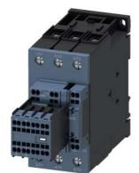
traction contactor, AC-3e/AC-3, 41 A, 18.5 kW / 400 V, 3-pole, 72 V DC, 0.7-1.25\* Us, electronic drive, with integrated varistor, auxiliary contacts: 2 NO + 2 NC, main circuit: screw terminal, control and auxiliary circuit: spring-loaded terminal, size: S2, removable auxiliary switch
