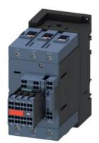
power contactor, AC-3e/AC-3, 80 A, 37 kW / 400 V, 3-pole, 24 V DC, 0.8-1.2\* Us, with integrated varistor, auxiliary contacts: 1 NO + 1 NC, integrated varistor, main circuit: screw terminal, control and auxiliary circuit: spring-loaded terminal, size: S3, suitable for PLC outputs, captive auxiliary switch
