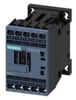
traction contactor, AC-1, 22 A, 400 V / 40 °C, 4-pole, 72-125 V DC, 0.7-1.25\* Us, electronic drive, with integrated varistor, auxiliary contacts: 1 NO + 1 NC, spring-loaded terminal, frame size: S00
