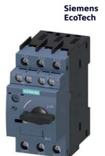
Special type Circuit breaker size S00 for motor protection, CLASS 10 A-release 4.5...6.3 A N-release 82 A screw terminal Standard switching capacity with transverse auxiliary switches 1 NO+1 NC Ambient temperature -50 °C 500 switching cycles
