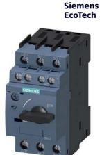
Special type Circuit breaker size S00 for motor protection, CLASS 10 A-release 9...12 A N-release 163 A screw terminal Standard switching capacity with transverse auxiliary switches 1 NO+1 NC Ambient temperature -50 °C 500 switching cycles
