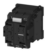
Contactor, Size 2, 2-pole, DC-3 and 5, 32 A Auxiliary contacts 22 (2NO + 2NC) 230 V AC 50/60 Hz AC operation Reusable packaging = 30 units
