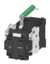
Contactor size 2, 2-pole for railway applications DC-3 and 5, 7.5 A at 750 V Auxiliary contacts 21 (2 NO + 1 NC) Operating range 0.7 to 1.25 x US connected to varistor DC magnet system 24 V DC Upright mounting position
