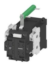
Contactor size 2, 2-pole for railway applications DC-3 and 5, 7.5 A at 750 V Auxiliary contacts 21 (2 NO + 1 NC) Operating range 0.7 to 1.25 x US connected to varistor DC magnet system 36 V DC Upright mounting position
