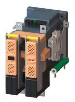
Contactor size 4, 2-pole DC-3 and 5, 75 A at 750 V Auxiliary contacts 21 (2 NO + 1 NC) Operating range 0.7 to 1.25 x US connected to varistor Direct current operation DC magnet system 24 V DC Mounting position vertical
