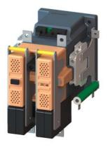
Contactor size 4, 2-pole DC-3 and 5, 75 A at 750 V Auxiliary contacts 21 (2 NO + 1 NC) Operating range 0.7 to 1.25 x US connected to varistor Direct current operation DC magnet system 110 V DC Mounting position vertical
