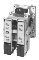
Contactor size 8, 2-pole DC-4, Rated operating current 220 A Auxiliary switch 22 (2 NO + 2 NC) Direct current operation G drive with integrated varistor 24 V DC vertical mounting position
