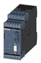
Basic unit SIMOCODE pro V PB, PROFIBUS DP interface 12 Mbps, RS485, 4I/3O freely parameterizable, US: 110...240 V AC/DC, Input for thermistor connection monostable relay outputs, with coated printed circuit boards, expandable by extension modules
