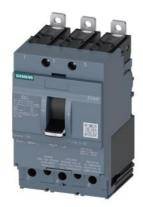
molded case switch 3VA4 UL frame 125 max short-circuit curr. rating 65kA @ 480 V 3-pole MCS110, In=100A without overload protection - self protection li=16 x In
