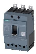
circuit breaker 3VA4 UL Frame 125 breaking capacity class S 25 kA @ 480 V 3-pole, line protection TM210, FTFM, In=110 A overload protection Ir=110 A permanently set short-circuit protection Ii=10 x In
