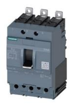
circuit breaker 3VA4 UL Frame 125 breaking capacity class M 35 kA @ 480 V 3-pole, line protection TM210, FTFM, In=125 A overload protection Ir=125 A permanently set short-circuit protection Ii=10 x In
