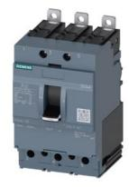
circuit breaker 3VA4 UL Frame 125 breaking capacity class H 65 kA @ 480 V 3-pole, line protection TM210, FTFM, In=125 A overload protection Ir=125 A permanently set short-circuit protection Ii=10 x In
