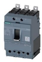
circuit breaker 3VA4 UL Frame 125 breaking capacity class S 25 kA @ 480 V 3-pole, line protection TM210, FTFM, In=20 A overload protection Ir=20 A permanently set short-circuit protection Ii=15 x In
