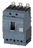
circuit breaker 3VA4 UL Frame 125 breaking capacity class S 25 kA @ 480 V 3-pole, line protection TM210, FTFM, In=30 A overload protection Ir=30 A permanently set short-circuit protection Ii=10 x In
