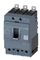
circuit breaker 3VA4 UL Frame 125 breaking capacity class M 35 kA @ 480 V 3-pole, line protection TM210, FTFM, In=30 A overload protection Ir=30 A permanently set short-circuit protection Ii=10 x In
