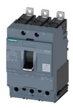
circuit breaker 3VA4 UL Frame 125 breaking capacity class H 65 kA @ 480 V 3-pole, line protection TM210, FTFM, In=30 A overload protection Ir=30 A permanently set short-circuit protection Ii=10 x In
