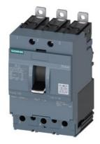
circuit breaker 3VA4 UL Frame 125 breaking capacity class H 65 kA @ 480 V 3-pole, line protection TM210, FTFM, In=35 A overload protection Ir=35 A permanently set short-circuit protection Ii=10 x In
