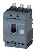
circuit breaker 3VA4 UL Frame 125 breaking capacity class S 25 kA @ 480 V 3-pole, line protection TM210, FTFM, In=70 A overload protection Ir=70A permanently set short-circuit protection Ii=10 x In
