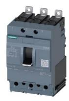
circuit breaker 3VA4 UL Frame 125 breaking capacity class S 25 kA @ 480 V 3-pole, line protection TM210, FTFM, In=15 A overload protection Ir=15 A permanently set short-circuit protection Ii=20 x In
