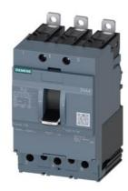
circuit breaker 3VA4 UL Frame 125 breaking capacity class H 65 kA @ 480 V 3-pole, line protection TM210, FTFM, In=15 A overload protection Ir=15 A permanently set short-circuit protection Ii=20 x In
