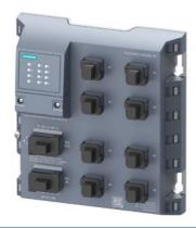
SCALANCE XP208G PP, managed layer 2 IE switch, 8x10/100/1000 Mbps, AIDA push/pull ports, IP65, -40 °C to +70 °C, power supply in/out, LED diagnostics, PROFINET IO device, network management, can be operated in redundant ring, dust caps, C-PLUG optional
