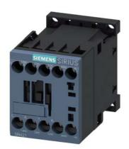
contactor relay, 2 NO + 2 NC, 24 V AC, 50/60 Hz, screw terminal, frame size S00, multi-unit packaging, pack = 40 units
