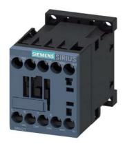
contactor relay, 2 NO + 2 NC, 125 V DC, screw terminal, frame size S00, reusable packaging, pack = 144 units
