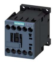
coupling contactor relay, 2 NO + 2 NC, 24 V DC,  $0.85-1.85^*$  Us, with integrated diode, screw terminal, frame size S00, multi-unit packaging, pack = 40 units
