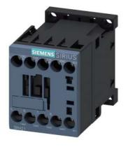
coupling contactor relay, 2 NO + 2 NC, 24 V DC,  $0.85-1.85^*$  Us, with integrated diode, screw terminal, frame size S00, reusable packaging, pack = 72 units
